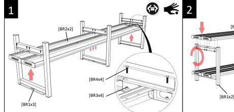
Lay the 3 main frames/legs [BR1] upside down. Place the 2 lower planks [BR1] within the frames and hold them evenly. Attach the legs to the planks, by using hex head bolts [BR3] and locknuts [BR4].
