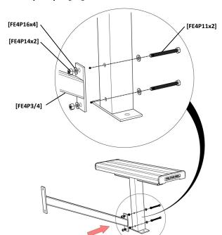
Secure the 4 assembled components achieved in the step 3, to the central post [FE4P1], by using hex. head bolts [FE4P10], locknuts [FE4P14] and washers [FE4P16] - Finger tighten.
