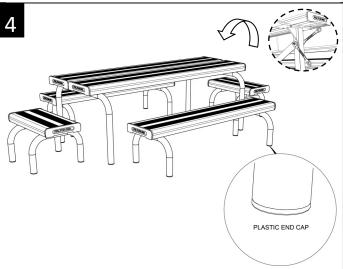
Tight the fasteners with spanners and appropriate tools.
