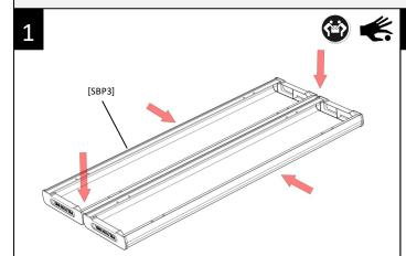
Lay 2 table planks **(SBP3)** upside down on a flat surface, making sure they are level at both ends.
