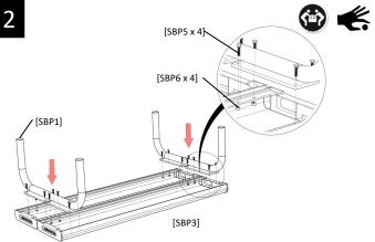
Bolt the two table frames/legs [SBP1] to the table planks [SBP3], by using hex. head bolts [SBP6] and locknuts [SBP7] - finger tighten.
