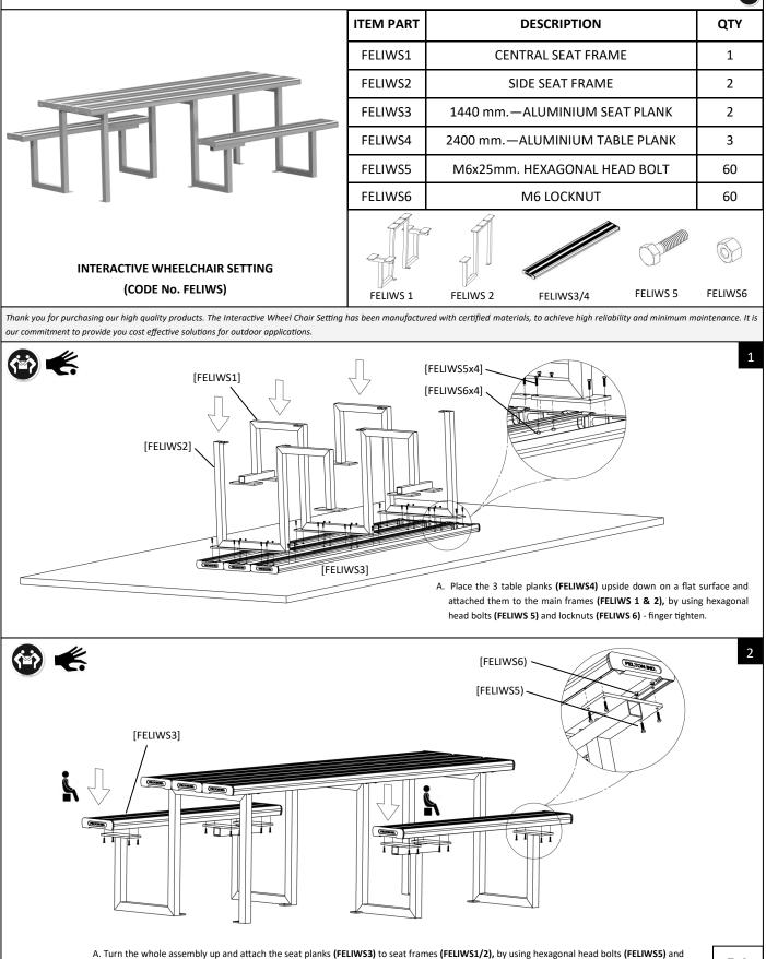
locknuts (FELIWS6) as indicated in the illustration above - finger tighten.
