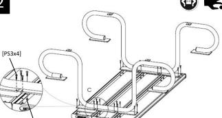
Lay 3 Aluminium planks (PS2) upside down on a flat surface, making sure they are level at both ends.
