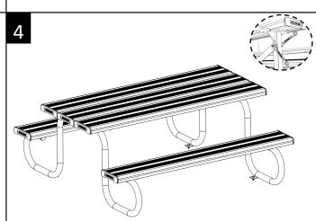
$\label{thm:continuous} \textbf{Tighten all hexagonal head bolts with spanners and appropriate tools.}$
