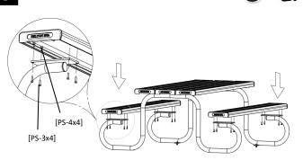
Turn the entire assembly up and install two seat planks (PS2) on to frame fixing plates as illustrated. Attach the seat planks (PS2) with hexagonal bolts (PS3) and nuts (PS4).
