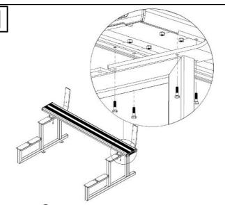
by using bolts **6** and nuts **7**. Note that all fixing lugs on base frames **①** face inwards.
