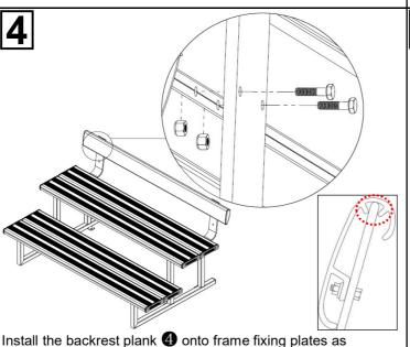
illustrated. Fasten the backrest planks **4** with hexagonal bolts
