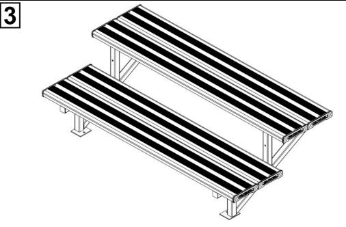
Attach the whole assembly in step 2 firmly to the ground and wall with appropriate dynalbolts M12 on each frame lug. Tighten all hexagonal head bolts with spanners and appropriate tools.
