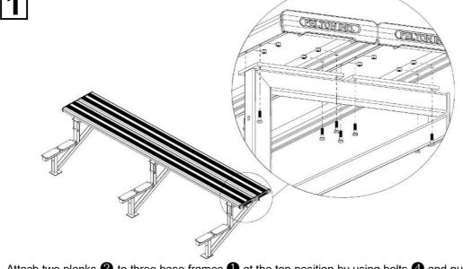
Attach two planks 2 to three base frames 1 at the top position by using bolts 4 and nuts 5. Note that all fixing lugs on base frames **1** face inwards.
