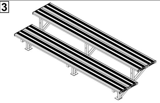
Attach the whole assembly in step 2 firmly to the ground and wall with appropriate dynalbolts M12 on each frame lug. Tighten all hexagonal head bolts with spanners and appropriate tools.
