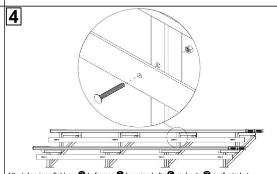
Attach two long flat bars **3** to frames **1** by using bolts **6** and nuts **7** as illustrated Ensure all bolts and nuts are tightened completely. The grandstand is now ready to be used!
