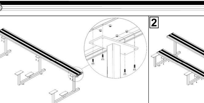
Attach one plank 2 to three base frames 1 at the top position by using bolts 3 and nuts 4 as illustrated. Note that all fixing lugs on base frames 1 face inwards.
