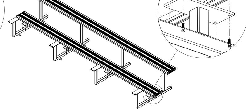
Attach another plank (2) to four base frames (1) at the lower position by using bolts (3) and nuts (4) as illustrated.
