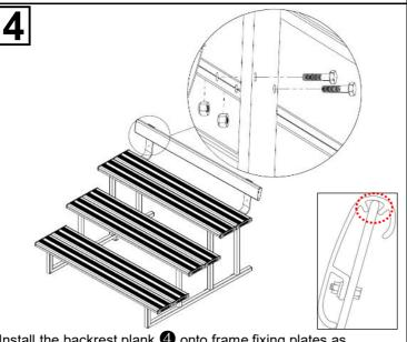
Install the backrest plank 4 onto frame fixing plates as illustrated. Fasten the backrest planks **4** with hexagonal bolts 6 and nuts 7. Ensure the fixing plates are installed in the right
