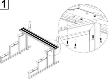
Attach plank 2 (with notch cut beneath) to two base frames 1 by using bolts 6 and nuts 7. Note that all fixing lugs on base frames **①** face inwards.
