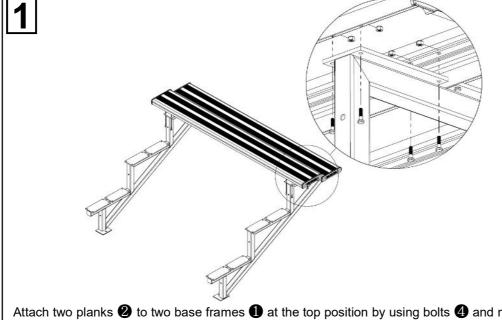
Attach two planks 2 to two base frames 1 at the top position by using bolts 4 and nuts 5. Note that all fixing lugs on base frames **1** face inwards.
