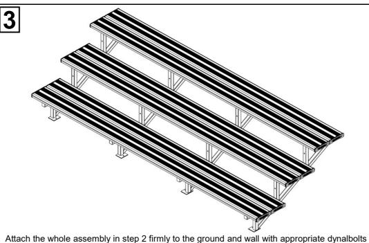
Attach three long flat bars **3** to frames **1** by using bolts **6** and nuts **7** as illustrated M12 on each frame lug. Tighten all hexagonal head bolts with spanners and appropriate tools. Ensure all bolts and nuts are tightened completely. *The grandstand is now ready to be used!*
