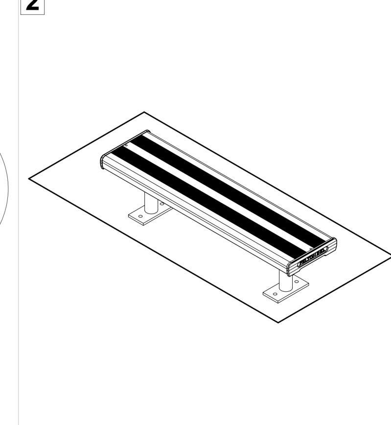
Attach the seat plank (2) to two leg supports (1) by using bolts (3) and nuts (4) as inllustrated.
