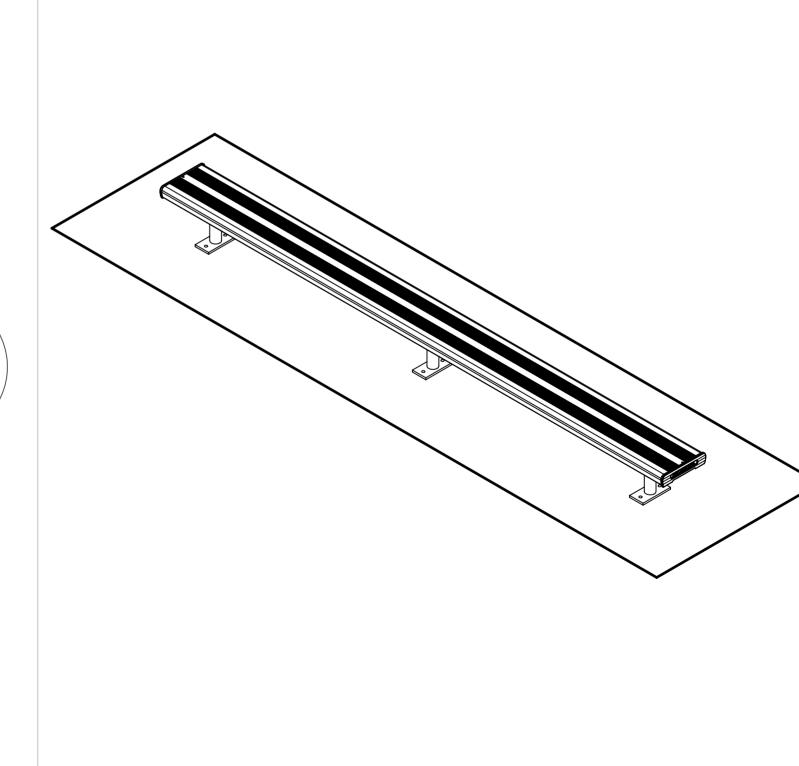
Tighten all hexagonal head bolts with spanners and appropriate tools. Then attach the whole assembly to the ground by using M12 dyna-bolts preferably, on each frame lug.
