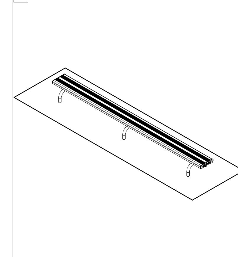
Tighten all hexagonal head bolts with spanners and appropriate tools. Then attach the whole assembly to the ground by using M12 dyna-bolts preferably, on each frame lug.
