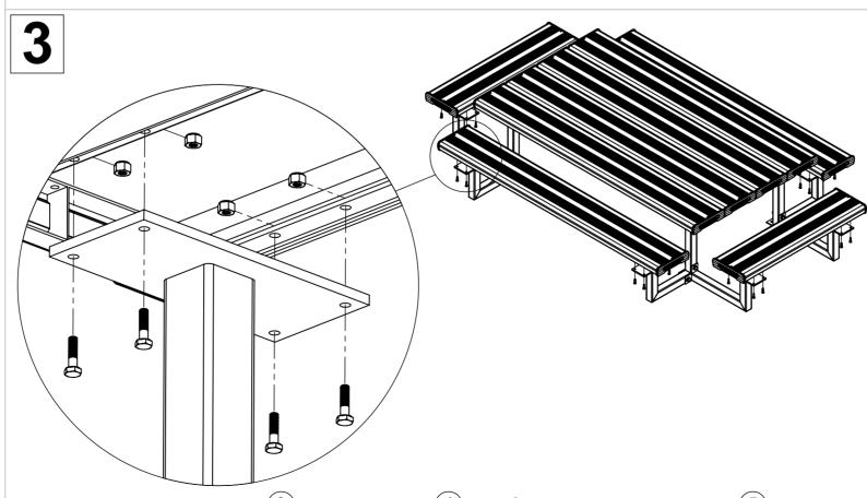
Attach two remaining planks (3) and two planks (4) onto fixing plates by using bolts (5) and nuts (6) as illustrated.
