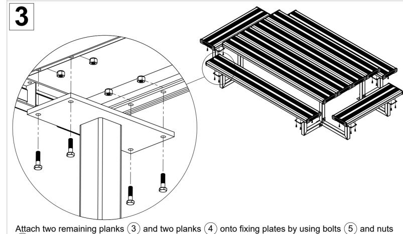
Tighten all hexagonal head bolts with spanners and appropriate tools. Then attach the whole assembly to the ground by using M12 dyna-bolts preferably, on each frame lug.
