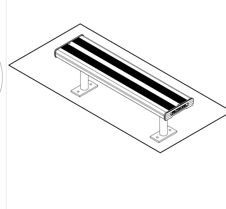
Tighten all hexagonal head bolts with spanners and appropriate tools. Then attach the whole assembly to the ground by using M12 dyna-bolts preferably, on each frame lug.
