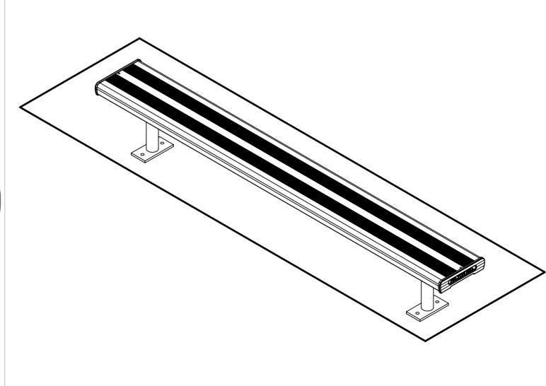
Tighten all hexagonal head bolts with spanners and appropriate tools. Then attach the whole assembly to the ground by using M12 dyna-bolts preferably, on each frame lug.
