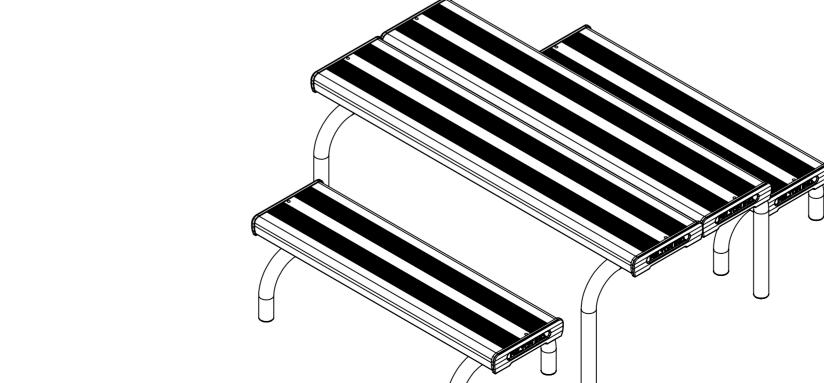
Tighten all hexagonal head bolts with spanners and appropriate tools. Then arrange all assemblies in previous steps as illustrated.
