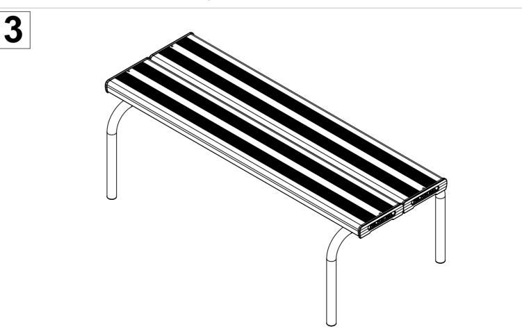
Tighten all hexagonal head bolts with spanners and appropriate tools. Then turn the assembly up.
