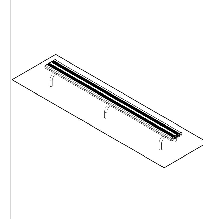
Tighten all hexagonal head bolts with spanners and appropriate tools. Then attach the whole assembly to the ground by using M12 dyna-bolts preferably, on each frame lug.
