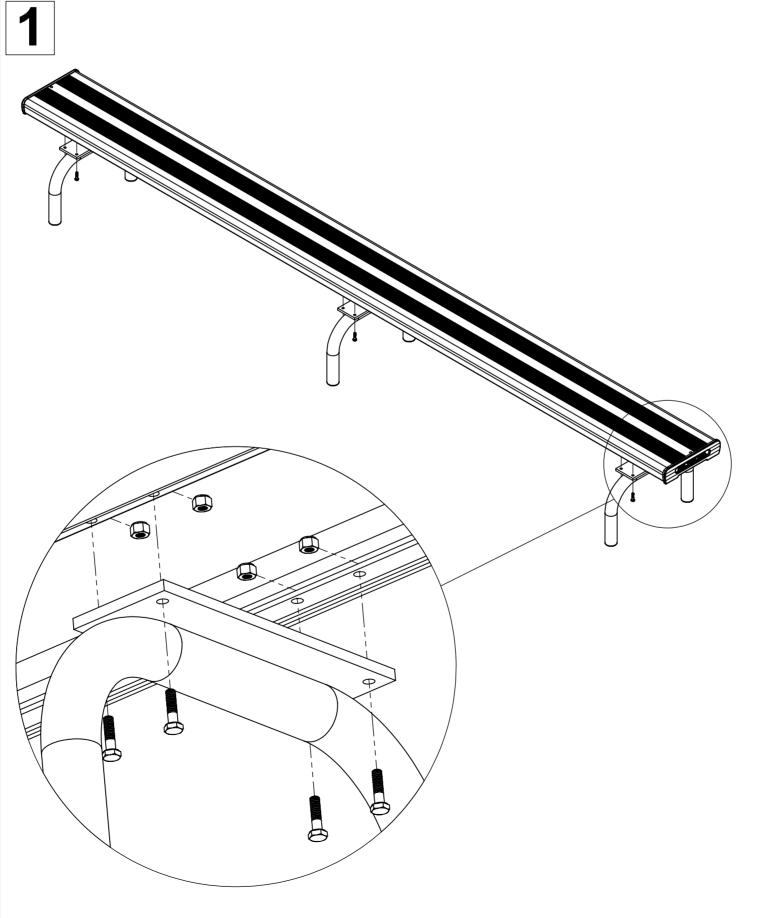
Attach the seat plank (2) to three leg supports (1) by using bolts (3) and nuts (4) as inllustrated.
