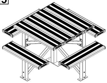
Tighten all hexagonal head bolts with spanners and appropriate tools. Then attach the whole assembly to the ground by using using M12 dyna-bolts preferably on each ground fixing plate.
