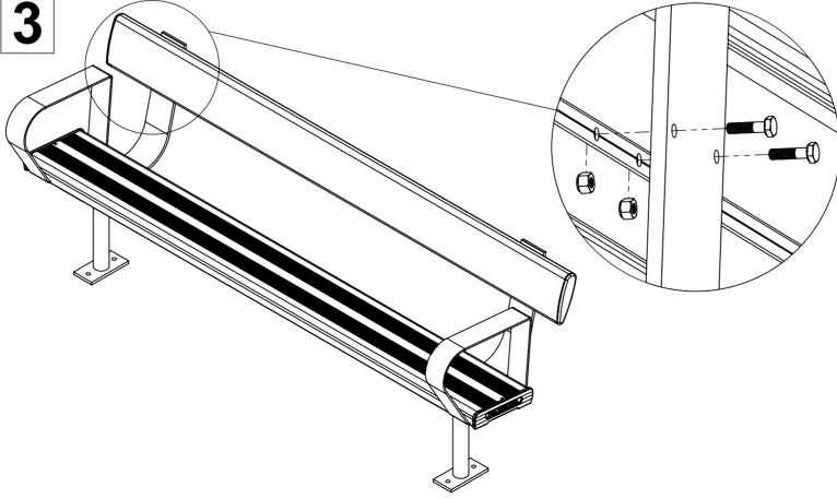
Attach the backrest plank (3) to the assembly in step 2 by using bolts (5) and nuts (6) as inllustrated.
