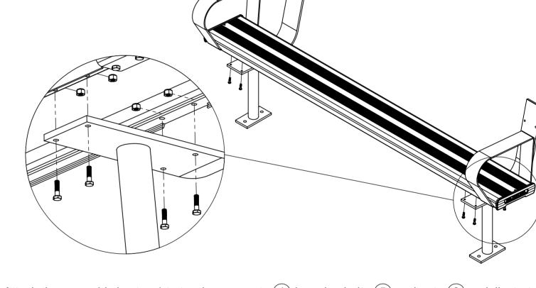
Attach the assembly in step 1 to two leg supports (1) by using bolts (5) and nuts (6) as inllustrated.
