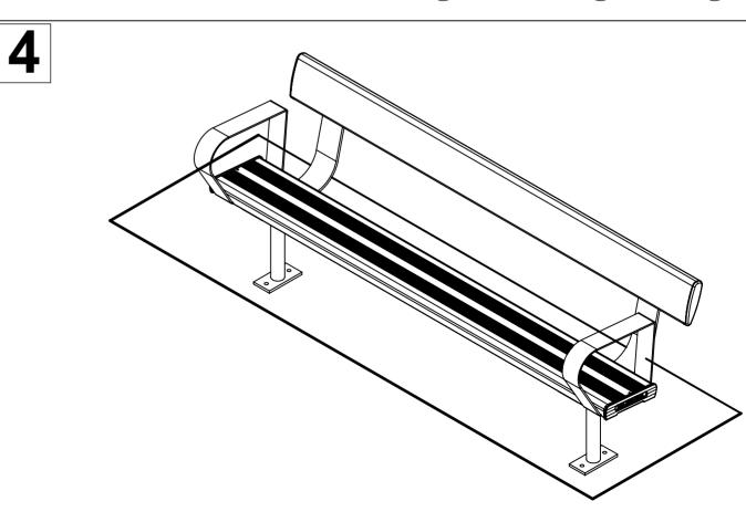
Tighten all hexagonal head bolts with spanners and appropriate tools. Then attach the whole assembly to the ground by using M12 dyna-bolts preferably, on each frame lug.
