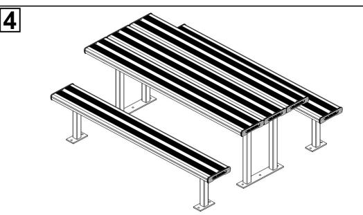
Tighten all hexagonal head bolts with spanners and appropriate tools. Then attach the table and seat assemblies to the ground by using M12 dyna-bolts on each ground fixing plate. Refer to the product's "SPECIFICATION DRAWING" for relative dimensions and technical recommendation.
