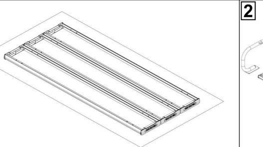
Place three planks 2 upside down and close together on the ground.
