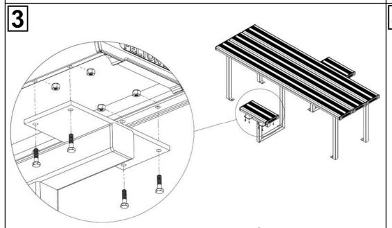
Turn the assembly in step 2 up, then attach two seat planks 4 onto fixing plates by using bolts **5** and nuts **6** as illustrated.
