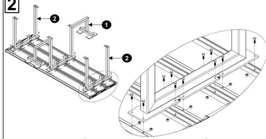
Attach central base frame 1 and two side frames 2 to three planks 3 in step 1 by using bolts 6 and nuts 6 as illustrated. Note that all fixing lugs on base frames 1 & 2 face inwards.
