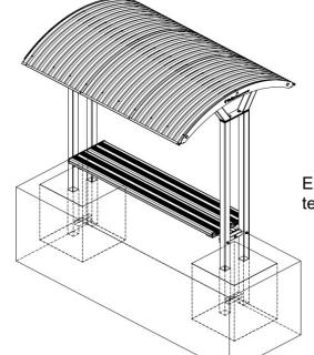
Embed the whole assembly to the concrete base as per technical recomendation in "SPECIFICATION DRAWING"
