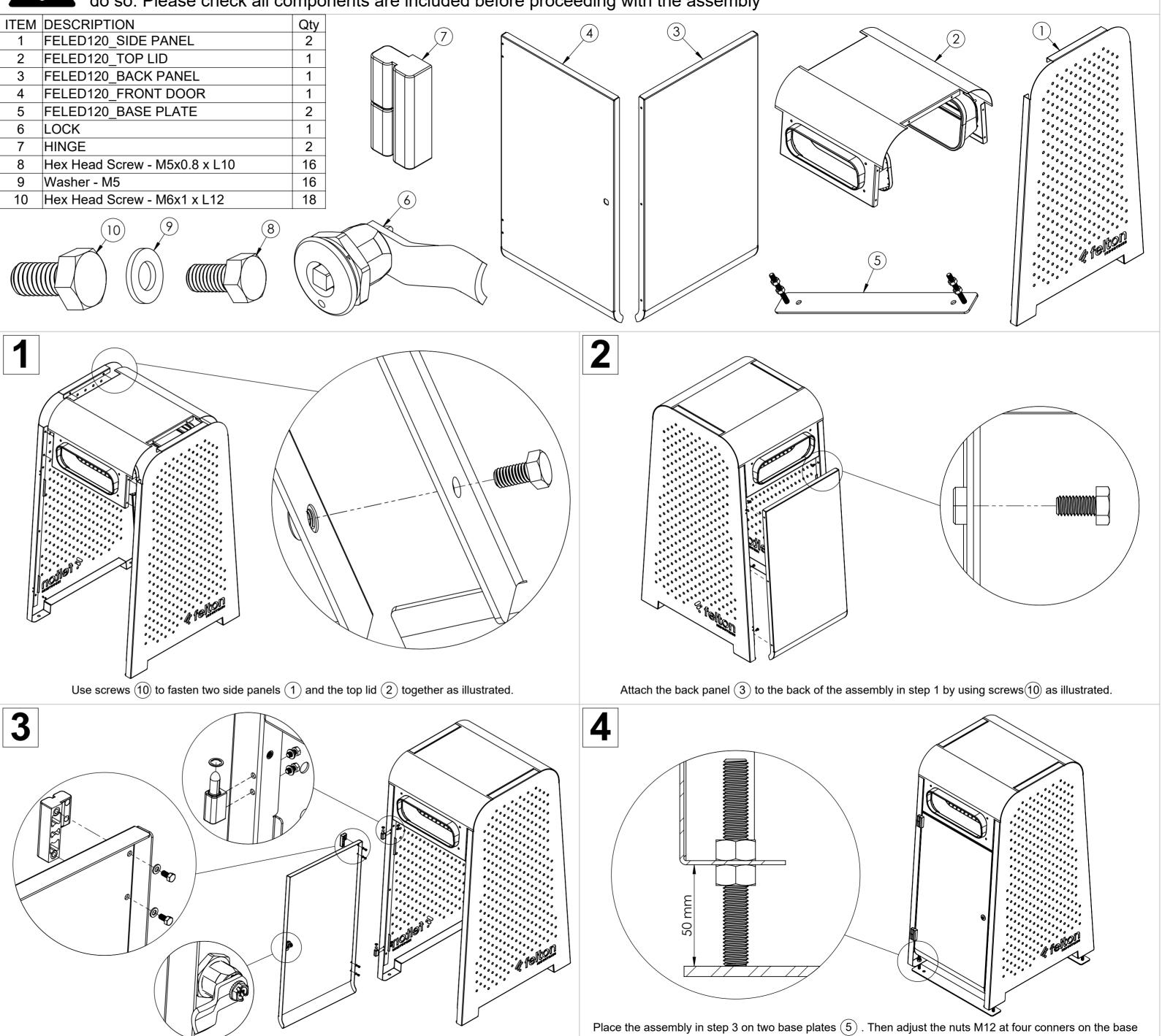
Attach two hinges (7) to the door panel (4) and the left side panel (1) by using screws (8) and washers (9) as illustrated. Then attach the lock (6) to the door panel (4)
