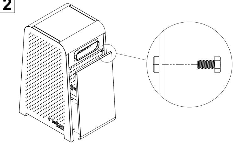
Use screws (10) to fasten two side panels (1) and the top lid (2) together as illustrated. Attach the back panel (3) to the back of the assembly in step 1 by using screws (10) as illustrated.
