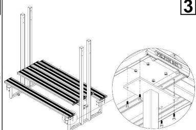
Install two seat planks **4** onto frame fixing plates as illustrated. Fasten the seat planks 4 with hexagonal bolts **(1)** and nuts **(11)**
