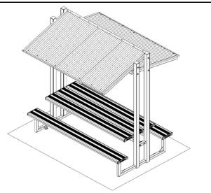
Tighten all hexagonal head bolts with spaners and appropriate tools. Then attach the whole assembly to the ground by using dyna-bolts preferably, on each frame lug
