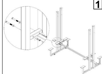
Attach the two main frames 1 and 2 to the connection bar 3 by using bolts 7, washes 8 and nuts **9**. Note that frame tags facing inward.
