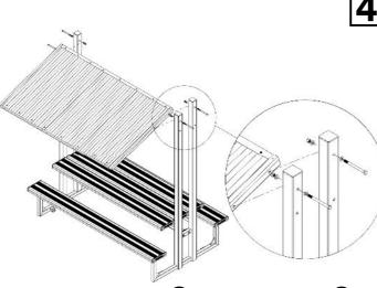
Attach the upper roof **6** to the main frame **1** and **2**. Fasten the upper roof **6** with hexagonal bolts 12, washers 8 and nuts 9
