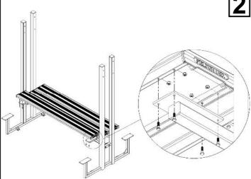
Install three table planks 6 onto frame fixing plates as illustrated. Fasten the table planks 6 with hexagonal bolts
