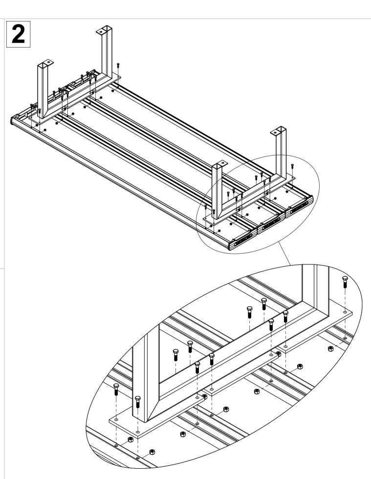
Attach two base frames (1) to three planks (2) in step 1 by using bolts (3) and nuts (4) as
