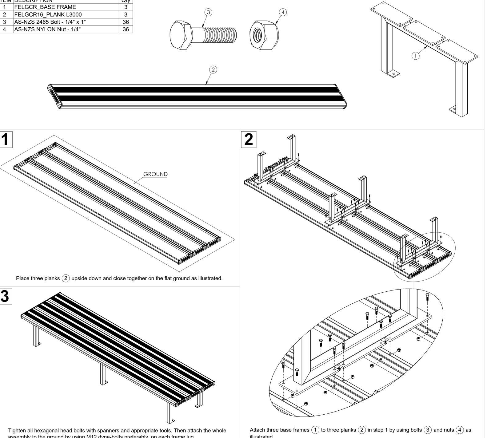
assembly to the ground by using M12 dyna-bolts preferably, on each frame lug.
