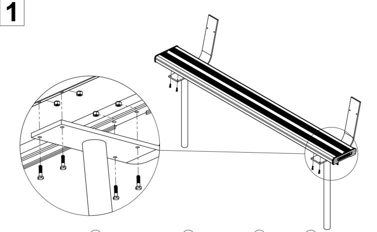
Attach the seat plank (2) to tow leg supports (1) by using bolts (4) and nuts (5) as inllustrated.
