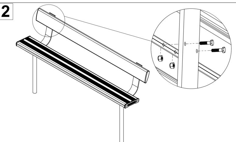
Attach the backrest plank (3) to the assembly in step 1 by using bolts (4) and nuts (5) as inllustrated.
