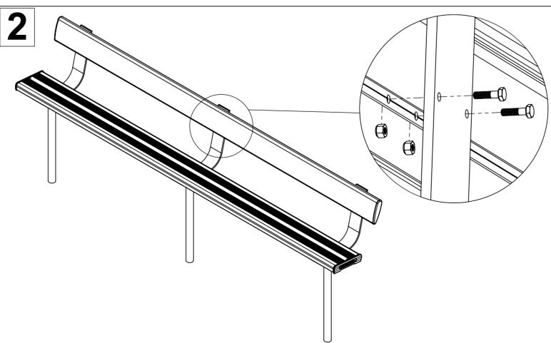
Attach the backrest plank (3) to the assembly in step 1 by using bolts (4) and nuts (5) as inllustrated.
