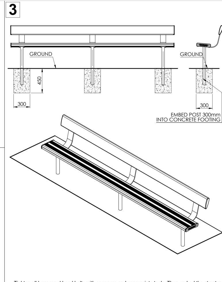
Tighten all hexagonal head bolts with spanners and appropriate tools. Then embed the structure min.300mm to the ground. Refer to "specification drawing" for detailed engineering requirement.
