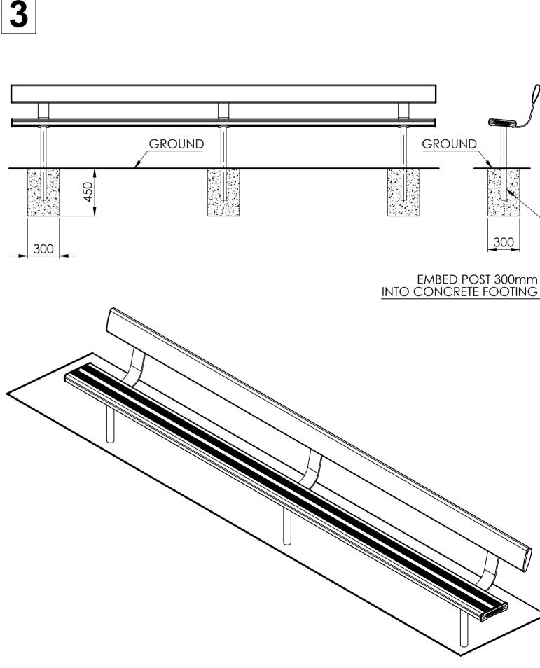
Tighten all hexagonal head bolts with spanners and appropriate tools. Then embed the structure min.300mm to the ground. Refer to "specification drawing" for detailed engineering requirement.
