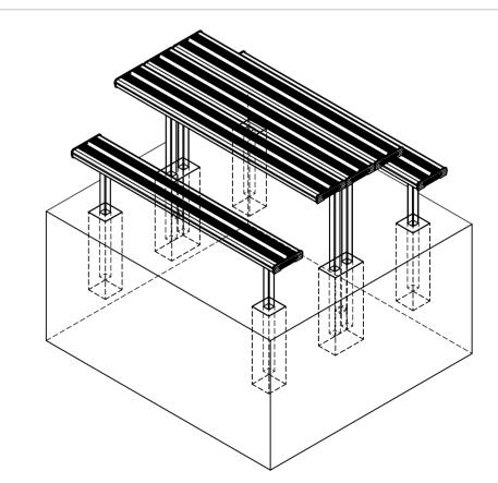
Tighten all hexagonal head bolts with spanners and appropriate tools. Then embed the table and seat assemblies 500 mm to the concrete bases as per technical recommendation in "SPECIFICATION DRAWING".
