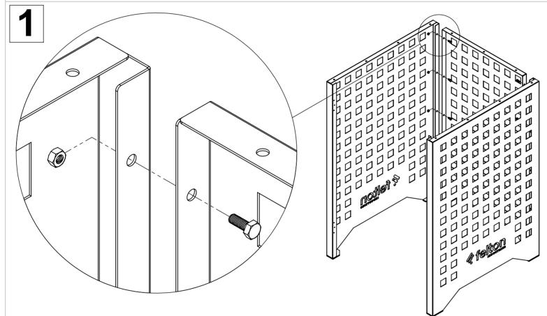
Attach the left side panel (2) and the right side panel (3) to the back panel (1) by using screws (9) and nuts (10) as illustrated.
