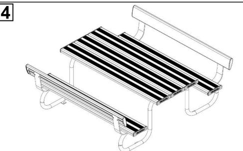
Tighten all hexagonal head bolts with spanners and appropriate tools. Then attach the whole assembly to the ground by using M12 dyna-bolts preferably, on each frame lug.
