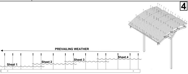
Fasten four corrugated roofs **4** to the assembly in step 3 by screws **9**. Ensure that the roofs' overlaping position and screws' position are conformed with the illustration in the picture. Note that the valleys of sheets should be turned-down at lower ends, and turned-up at upper ends as recommendation from manufacturer.
