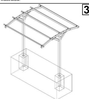
Embed the whole assembly 600 mm to the concrete base as per technical recommendation in "SPECIFICATION DRAWING"
