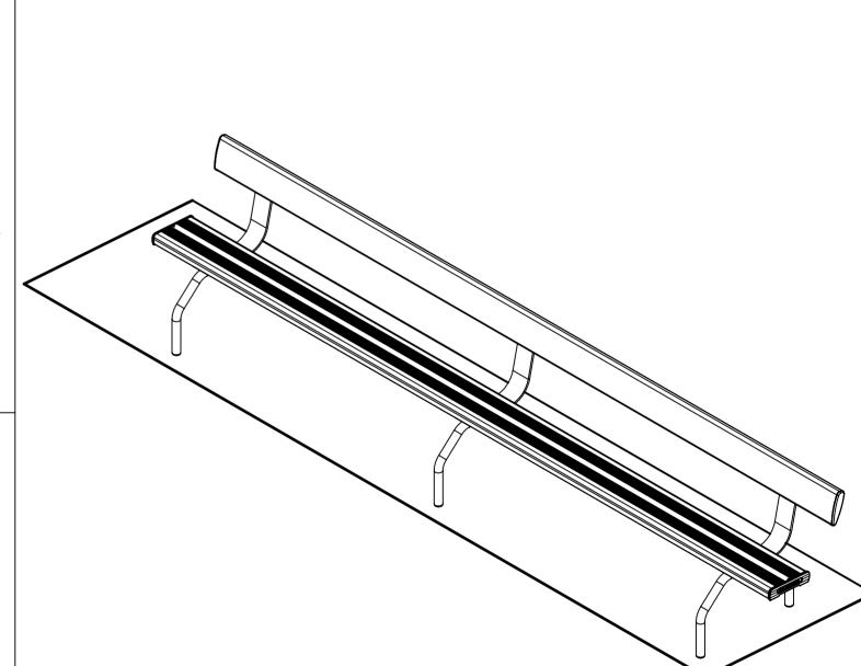
Tighten all hexagonal head bolts with spanners and appropriate tools. Then attach the whole assembly to the ground by using M12 dyna-bolts preferably, on each frame lug.
