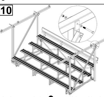
Attach two connection bars (19) to assembly in step 9 by using bolts 22, washers 12 and nuts 13 as illustrated.
