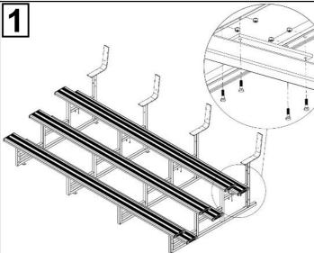
Attach six planks **2** to four base frames **1** to create tread and seat platforms by using bolts **7** and nuts **8**. Note that all fixing lugs on base frames face inwards.
