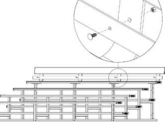
Attach the long flat bar **5** to fixing plates by using bolts **9** and nuts **()** as illustrated.
