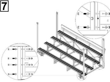
Attach two front roof frames (1) and two rear roof frames (1) to the assembly in step 6 by using bolts (1), washers (2) and nuts 13 as illustrated.
