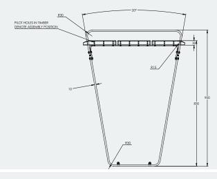
Dimensions of seat: 450mm D x 1924mm L x 520mm H Dimensions of shorter seat: 450mm D x 1060mm L x 520mm H
