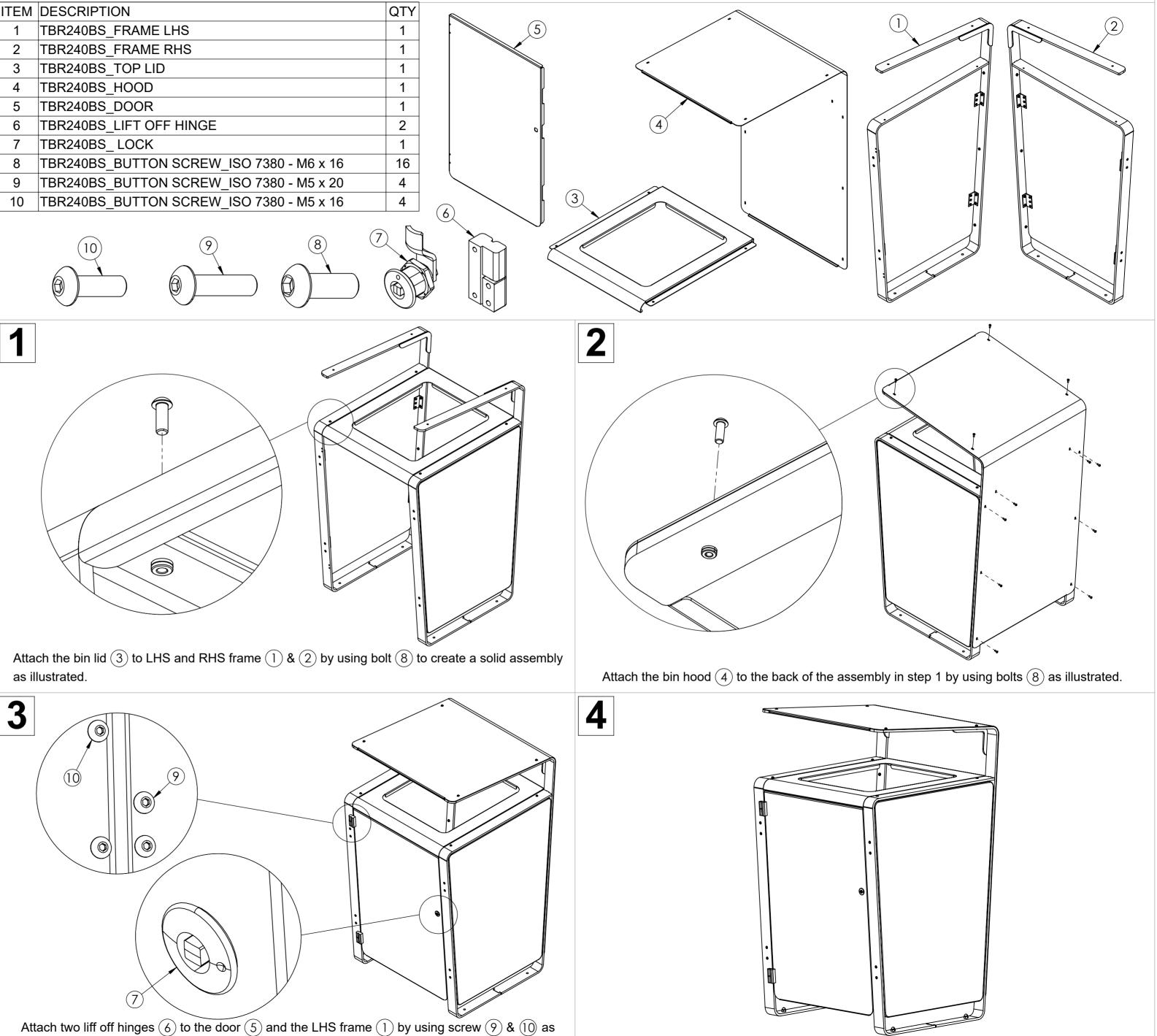
illustrated. Then attach the cam lock (7) to the door.
