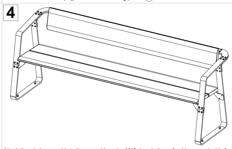
Attach the whole assembly to the ground by using M10 dyna-bolts preferably, on each side frame.
