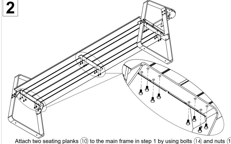
Attach two seating planks (10) to the main frame in step 1 by using bolts (14) and nuts (15) Then attach the strap 9 beneath two seating planks 10 as illustrated.
