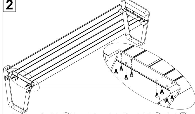
Attach two seating planks (5) to two main frames in step 1 by using bolts (7) and nuts (8) as illustrated.
