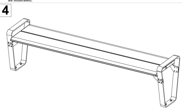
Attach the whole assembly to the ground by using M10 dyna-bolts preferably, on each side frame.
