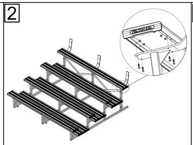
Attach 4th seat plank ③ (with notch cut beneath) to the assembly in step 1 by using bolts ⑦ and nuts ⑧ as illustrated.
