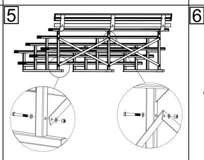
Attach four flat bars 6 to the back of base frames 1 by using bolts 1, washers 2 and nuts 3 as illustrated.
