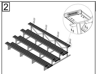
Attach 4th seat plank ③ (with notch cut beneath) to the assembly in step 1 by using bolts ⑦ and nuts ⑧ as illustrated.
