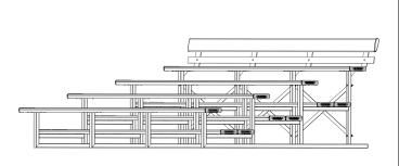
Tighten all hexagonal head bolts with spanners and appropriate tools. Then completely tighten the M12 dynabolts to attach the whole assembly firmly to the ground.
