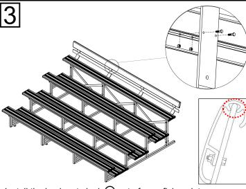
Install the backrest plank 4 onto frame fixing plates as illustrated. Fasten the backrest plank 4 with hexagonal bolts 7 and nuts 8. Ensure the fixing plates are installed in the right place on backrest plank.
