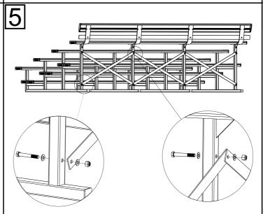
Attach six flat bars 6 to the back of base frames 1 by using bolts 1, washers 2 and nuts 3 as illustrated.
